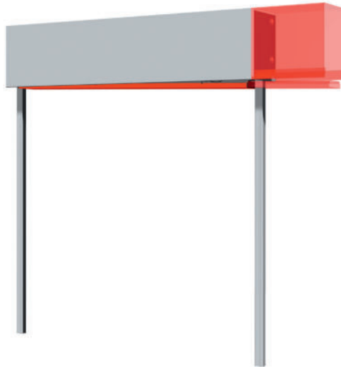
Figure 16: Changed limit position of the bottom rail (slanted bottom rail), slat stack visible on one side
