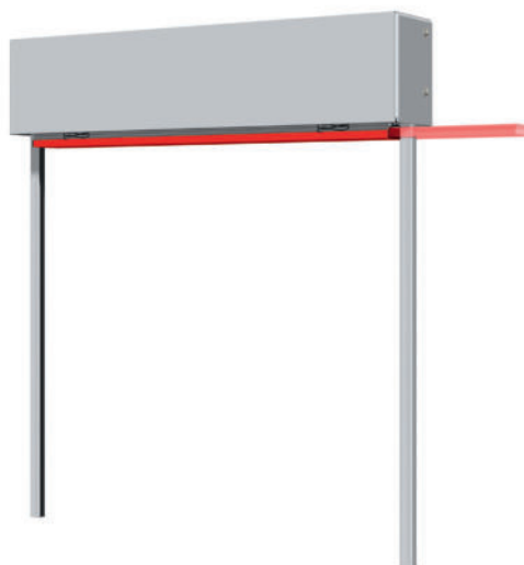
Figure 17: Changed limit position of the bottom rail (bottom rail is horizontal), slat stack is visible along its entire width
